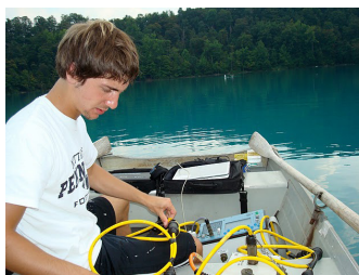
Nathan Barber, Geosciences undergrad, collects self potential data to map the location of the chemocline
