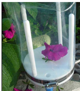
This picture shows the cuvette unit to study volatile emissions from flowers of different morphologies.
